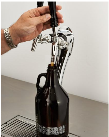
4. Insert filler tube into rinsed growler then pull handle forward to begin flow.
